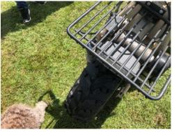
Standard feature are these chunky off-road tyres, on wheels that are an additional pair of tanks and can be used to carry extra fuel or even
